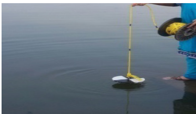
Figure 5: Check the transparency of water by using Secchi Disk.
