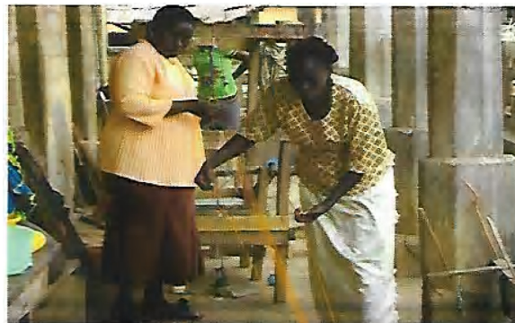
Figure 6: Draw in Warp Yarns on the Horizontal Loom.
