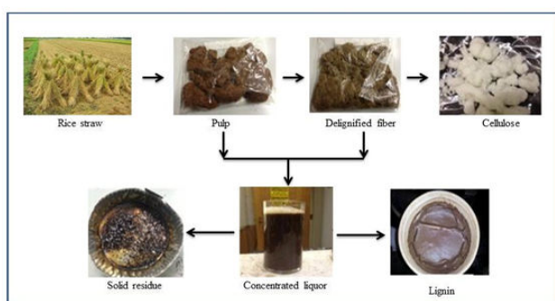
Figure 1: Schematic diagram of the process of lignin extraction
