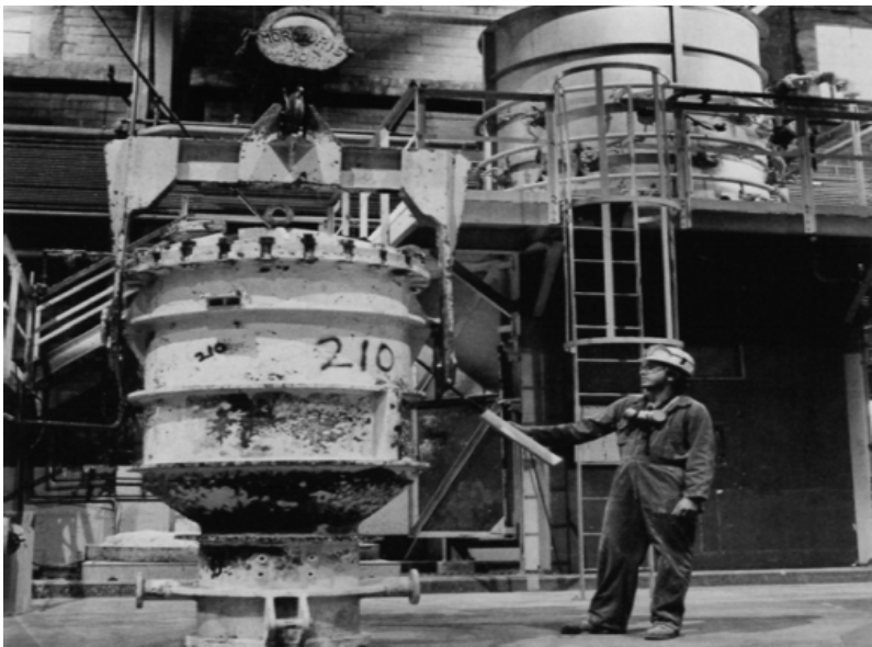
Figure 13: Large scale bomb for conducting a modern metallothermic reaction.
