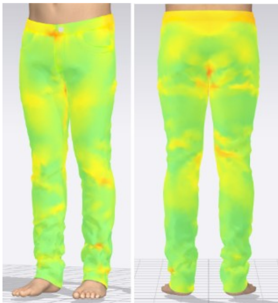
Figure 17: Stress map of the high stretch garment with 2% reduction in measurements (front and back).
