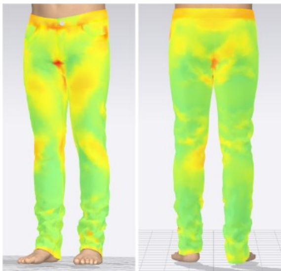
Figure 16: Stress map of the high stretch garment with 3% reduction in measurements (front and back).
