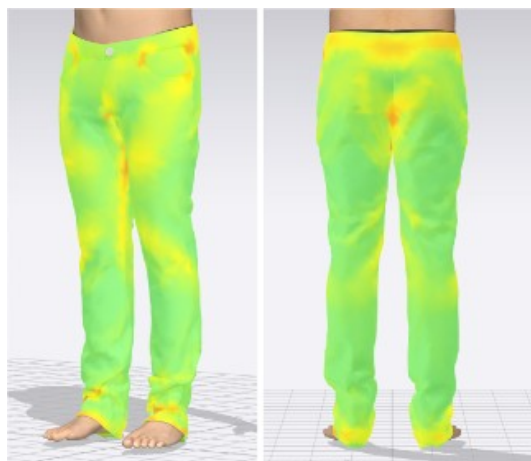
Figure 14: Stress map of the new garment created by CLO readings (front and back).
