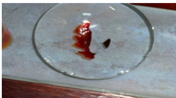
Figure 8: Aspect of the complex structured DCPD-GL complex film.
