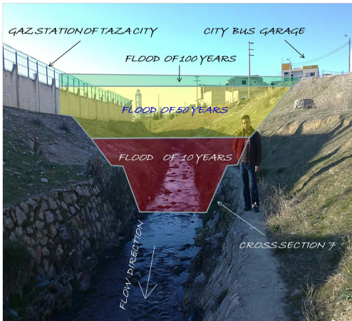
Figure 8: Possible flood spread scenario for different flood frequencies.
