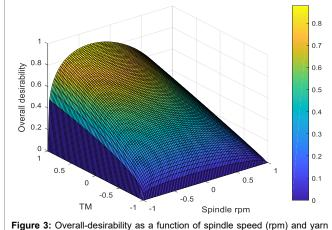
Figure 3: Overall-desirability as a function of spindle speed (rpm) and yarn twist (TM) for 10% shade depth blow room blended cotton mélange yarn.
