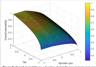
Figure 5: Overall-desirability as a function of spindle speed (rpm) and yarn twist (TM) for 40% shade depth draw frame blended cotton mélange yarn.
