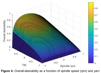
Figure 4: Overall-desirability as a function of spindle speed (rpm) and yarn twist (TM) for 70% shade depth blow room blended cotton mélange yarn.
