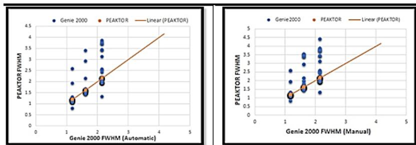
Figure 7: Comparison between PEAKTOR & Genie 2000 FWHM.
