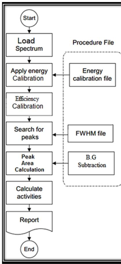
Figure 1: Flowchart for identification analysis.
