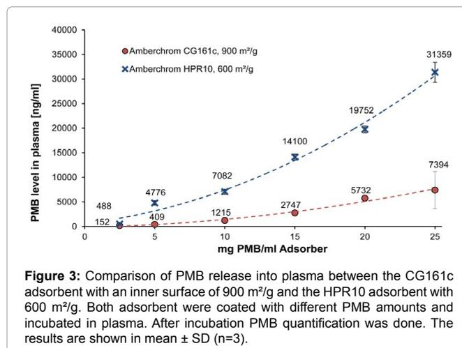
**Figure 3:** Comparison of PMB release into plasma between the CG161c adsorbent with an inner surface of 900 m<sup>2</sup>/g and the HPR10 adsorbent with 600 m<sup>2</sup>/g. Both adsorbent were coated with different PMB amounts and incubated in plasma. After incubation PMB quantification was done. The results are shown in mean ± SD (n=3).
