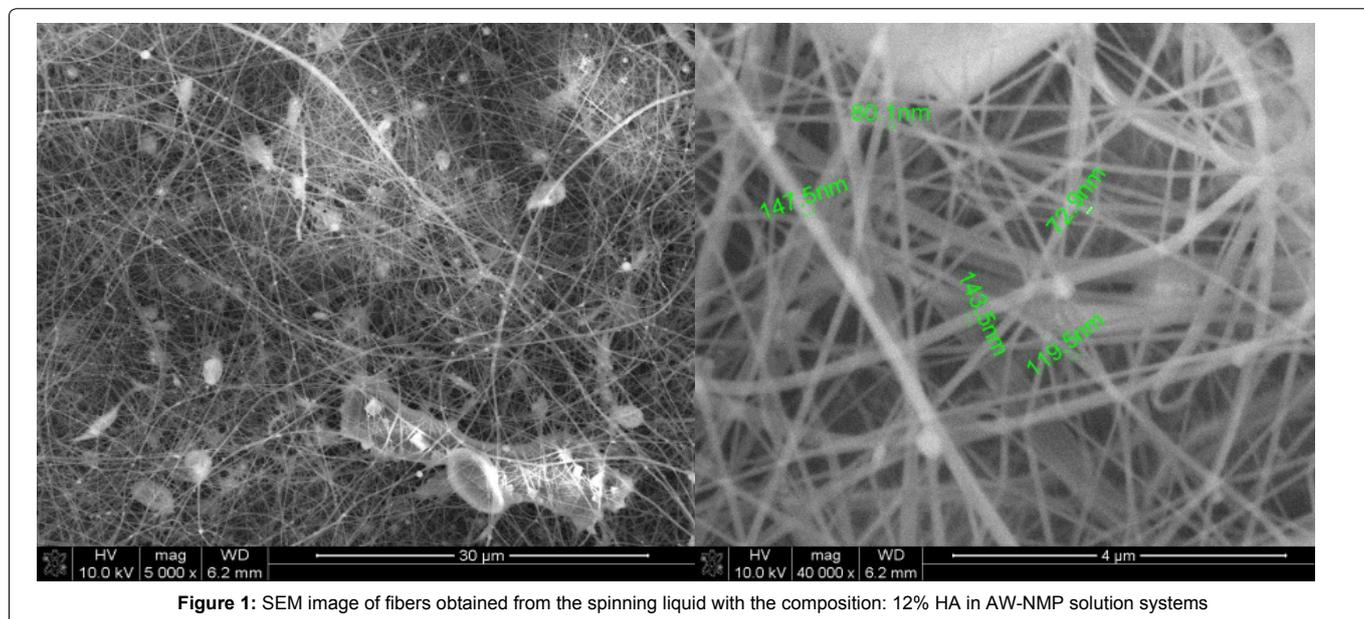
**Figure 1:** SEM image of fibers obtained from the spinning liquid with the composition: 12% HA in AW-NMP solution systems
