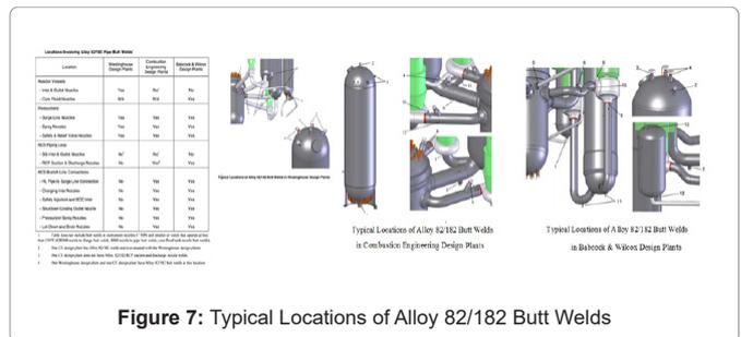
Figure 7: Typical Locations of Alloy 82/182 Butt Welds
