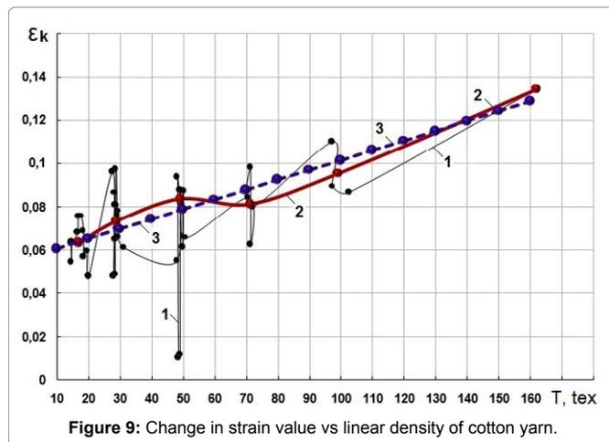
Figure 9: Change in strain value vs linear density of cotton yarn.
