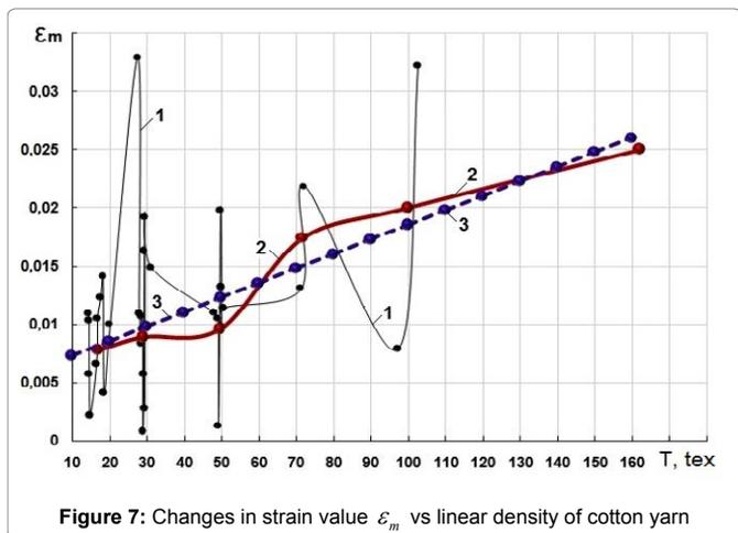
Figure 7: Changes in strain value  $\epsilon_m$  vs linear density of cotton yarn
