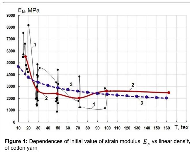
Figure 1: Dependences of initial value of strain modulus  $E_N$  vs linear density of cotton yarn
