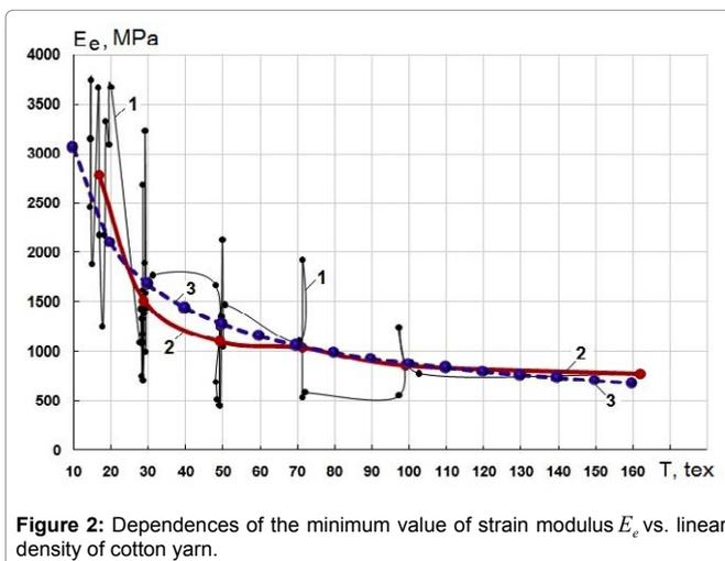
Figure 2: Dependences of the minimum value of strain modulus  $E_e$  vs. linear density of cotton yarn.
