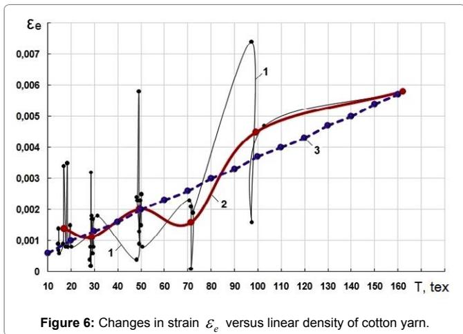
Figure 6: Changes in strain  $\epsilon_e$  versus linear density of cotton yarn.
