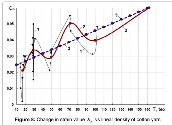
Figure 8: Change in strain value  $\epsilon_s$  vs linear density of cotton yarn.
