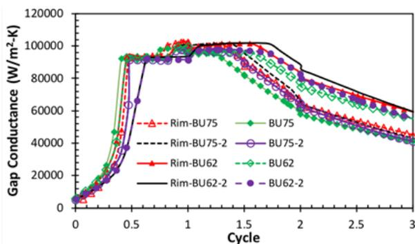
Figure 5: Gap conductance evolution as a function of cycle.
