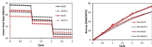
**Figure 2:** The left Figure shows the linear average power profile for three cycles. BU62/BU62-2 and BU75/BU75-2 are corresponding to 4.5-year normal and 6-year with burn up extension operation, respectively. The Figure on the right shows the burn up as a function of cycle number.
