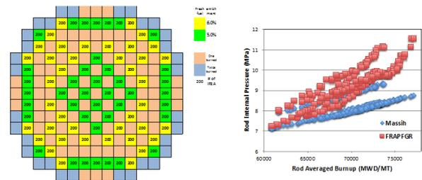
**Figure 1:** The left Figure on shows the loading map for a 24 months cycle design for a typical PWR and the Figure on the right show the comparison of calculated rod internal pressure with Massih and FRAPFGR models for all the fuel rods in a twice-burnt assembly with burn up extension.
