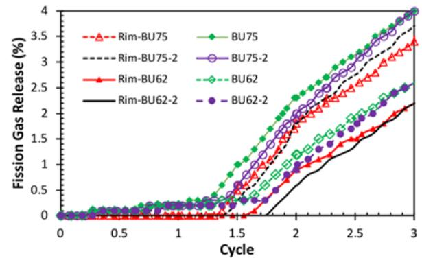
**Figure 3:** Fission gas release evolution as a function of cycle.
