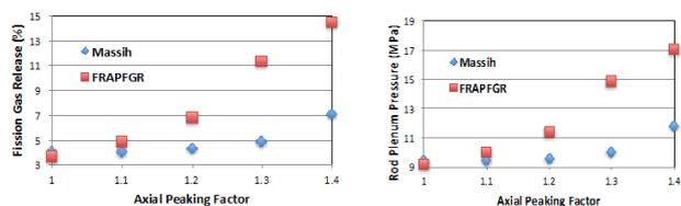
**Figure 6:** The left Figure shows the comparison of fission gas release for Massih and FRAPFGR models with different axial peaking factors. The Figure on the right shows the comparison of rod internal pressure for Massih and FRAPFGR models with different axial peaking factors.
