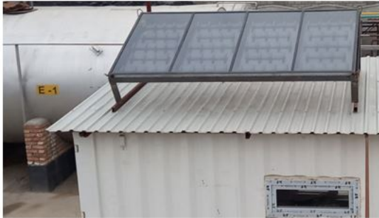
Figure 1: General view of a four-section solar air heater with concave air tube.
