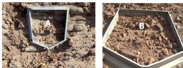
Figure 5: View of the runoff plots in the granite area: (A) Rocky area, (B) Colluvial area.
