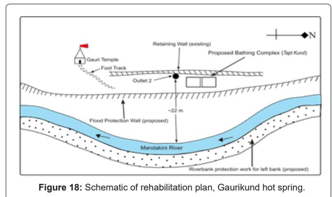
**Figure 18:** Schematic of rehabilitation plan, Gaurikund hot spring.
