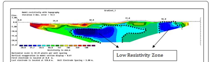
Figure 15: 2D ERT section along the profile line P1-P2-P3 using the Gradient configuration.
