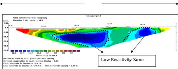
Figure 13: 2D ERT section along the profile line P1-P2-P3 using the Wenner configuration.
