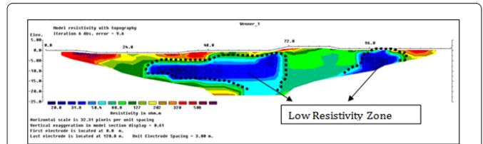
Figure 14: 2D ERT section along the profile line P1-P2-P3 using the Schumberger configuration.
