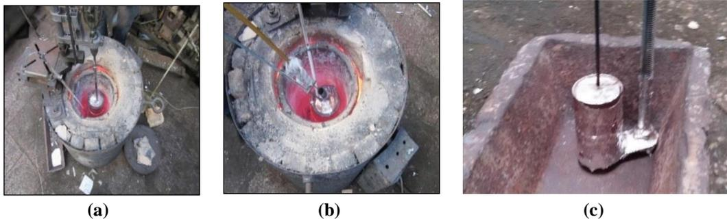
**Figure 2:** (a): Homogenization of the melt; (b): Taking a sample; (c): A cast sample together with the mould.
