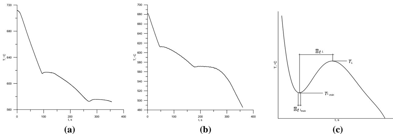
**Figure 3:** (a): Dependence of the temperature on time for sample S1 without NC; (b): Dependence of the temperature on time for sample S6N with NC 0.05 wt% TiN; (c): Scheme for determining the quantities of the temperature dependencies.
