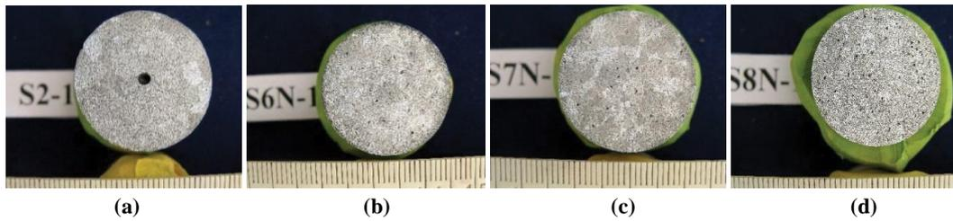
**Figure 4:** Macrostructures of samples-without and with NC (a): S2-1-without NC; (b): S6N-1-1part TiN+1.5 parts Cu, 0.05 wt% TiN; (c): S7N-1-composite rod: 4 $\mu$ .SiC+1 $\mu$ .Cu+12 $\mu$ .Al, 0.05 wt% SiC; (d): S8N-1-1 part TiCN+2 partsTi, 0.04 wt% TiCN.
