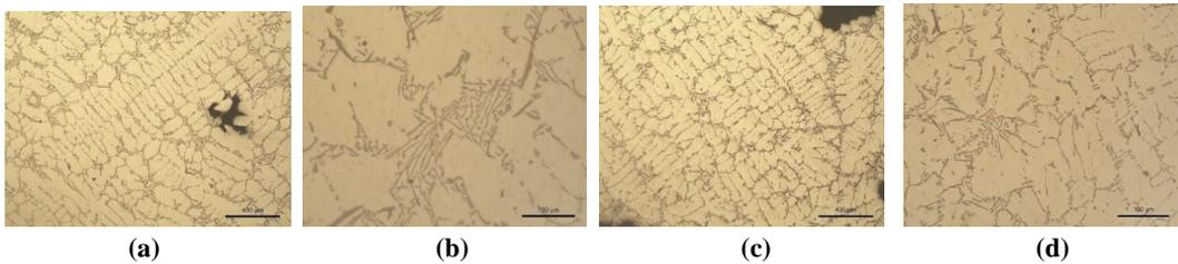
**Figure 5:** Microstructure of samples S2-1 and S8N-1 (a): general view of the microstructure of sample S2-1; (b): eutectic in sample S2-1; (c): general view of the microstructure of sample S8N-1; (d): eutectic in sample S8N-1.
