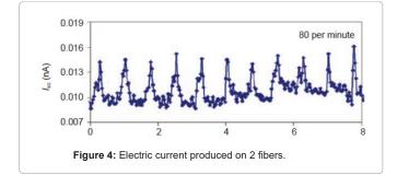
The twist of the nanowires create output current during a cyclic comparative slide between both the two strands Figure 4. The fiberbased nanogenerator [25-31] can harvest energy *via* body movement, muscular stretch, gentle breeze, and vibrations.
