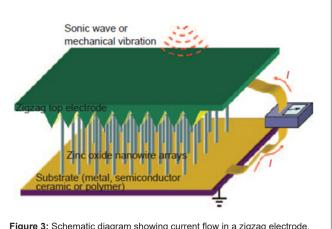
Figure 3: Schematic diagram showing current flow in a zigzag election
