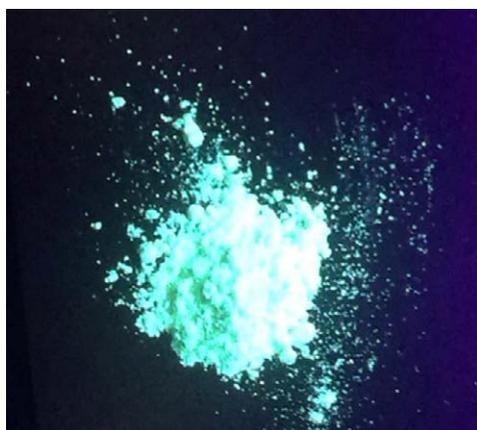
Figure 2: The fluorescent of the synthesized powder under UV excitation at 366 nm wavelength.
