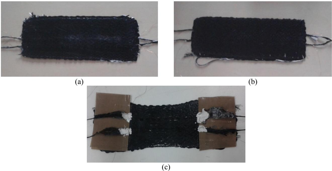
Figure 3: Textile reinforced 2D thermoplastic composites with integrated textile sensors developed by 2D textile preforms consolidation condition I: (a) case I, (b) case II, (c) case III.
