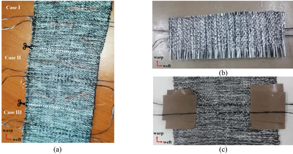
Figure 2: Textile sensors: (a) integration during weaving of 2D fabric, (b) 2D textile preform preparation for thermal consolidation - case I and II, (c) 2D textile preform preparation for thermal consolidation - case III.
