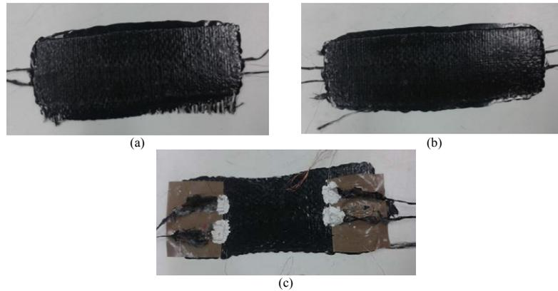
**Figure 4:** Textile reinforced 2D thermoplastic composites with integrated textile sensors developed by 2D textile preforms consolidation condition II: (a) case I, (b) case II, (c) case III.
