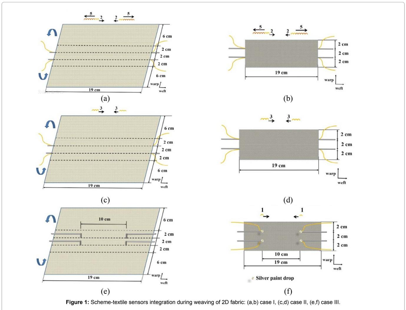
Figure 1: Scheme-textile sensors integration during weaving of 2D fabric: (a,b) case I, (c,d) case II, (e,f) case III.
