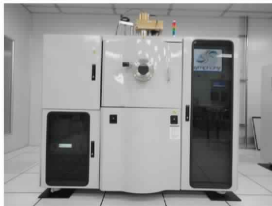
Figure 1: Tecport Sputter Coater used for coating stainless steel wires with titanium oxide coating.
