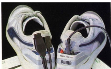
Figure 2: Puma RS (Running System) computer-connected shoes (URL_8).
