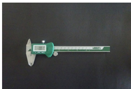
Figure 1: Vernier caliper with 0.01 mm.
