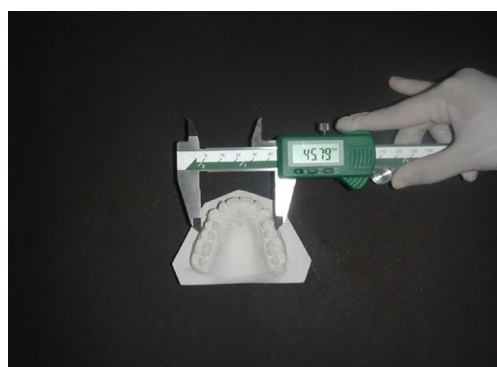
Figure 3: Measuring inter-premolar width at Table1 in study model.
