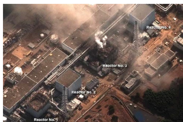
Figure 1: Fukushima Daiichi nuclear disaster: Fukushima damaged reactors. In this photograph, smoke escapes from the roof of reactor No. 3 which has just been blown by an explosion, forty hours after the one that happened on unit 1. The explosion that was to occur on reactor No. 2 has yet to come. These non-explosions, but hydrogen explosions due to large amounts of hydrogen produced by the prolonged absence of cooling, and that leaked and mixed with air. Source: Japan Atomic Industrial Forum, Tepco.
