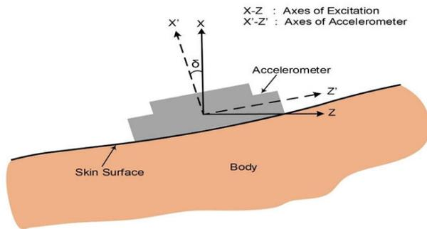
**Figure 3:** Illustration of accelerometer axes attached to the body relative to the excitation/platform axes.
