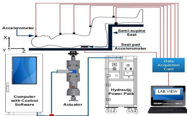
**Figure 1:** Schematic representation of vibration simulator.
