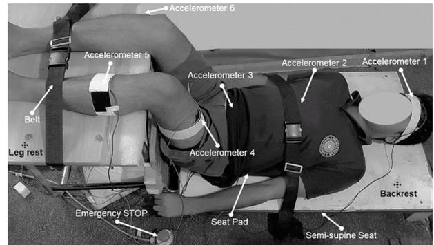
**Figure 2:** Subject lying on a semi-supine seat. The vibration signals were acquired using five accelerometers attached to the body at the head (1), sternum (2), abdomen (3), thigh (4), and leg (5). The semi-supine seat vibration was measured at the backrest by the seat pad accelerometer (beneath the subject) and the leg rest by an accelerometer (6).
